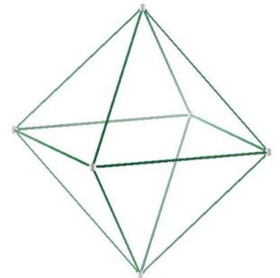
**Hint:** Consider a plane of symmetry half way between the two edges, A and B. Each point where it intersects the octahedron, has the same voltage (which is the average of the voltages in A and B). If we now connect all those points together, this will not change the resistance of the circuit (since no current would flow between the points at equal voltages).
