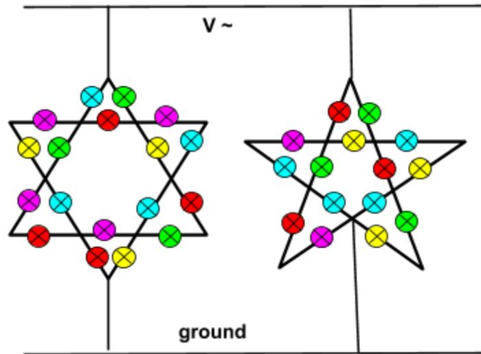
**Hint:** For a given voltage  $V$ , power  $P = V^2/R$ , where  $R$  is the total resistance of the circuit.
