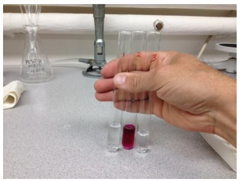
Then I washed all three test tubes, and poured fresh solutions "1", "2", or "3" to each of them. As previously, the number on the bottle corresponded to the test tube number. After that, I added a solution "1" to the solutions "2" and "3", and I observed formation of precipitates in the tube "2", and "3":
