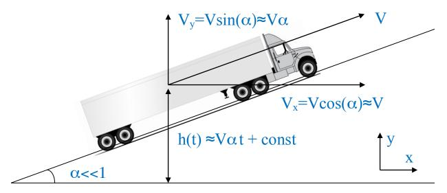
The potential energy of the truck (of mass m including the cargo of mass M) could be written as
