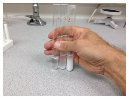
Then I washed test tubes again, and added the solution "3" to the solutions "1" and "2". Only a solution "1" gave a precipitate with a solution "3"; no precipitation was observed in the test tube "2":
