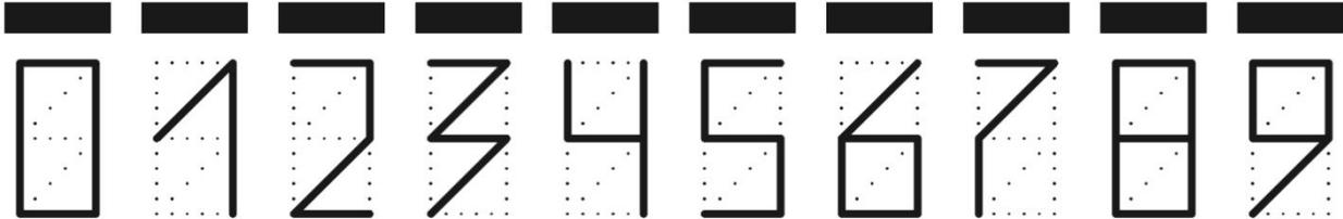
The system checked one of the 9 intervals (2 diagonal, 6 on the outside of the box, 1 horizontal interval inside the box) to determine whether it is filled out or not. In order to determine which digit is written, the system had to be programmed to check a certain set of these intervals, and based on the result of these checks, it had to determine which digit was written.
