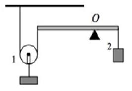
**Hint:** Apply the law of the lever. The plank's gravity force is applied to its center of mass. The tension of the rope at pulley is half of the weight of  $m_1$ .
