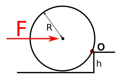
**Hint:** Imagine that the cylinder had just detached from the floor. Sketch all the forces acting on it. In order for it to roll over, the net torque acting on the cylinder, *with respect to the point O*, should be directed clockwise.
