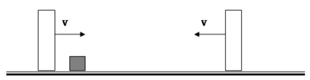
Two very massive walls are moving toward each other with identical speeds V. A light box is initially resting on a frictionless surface between the two walls as shown. Find the speed of the block after three elastic collisions with the walls.
