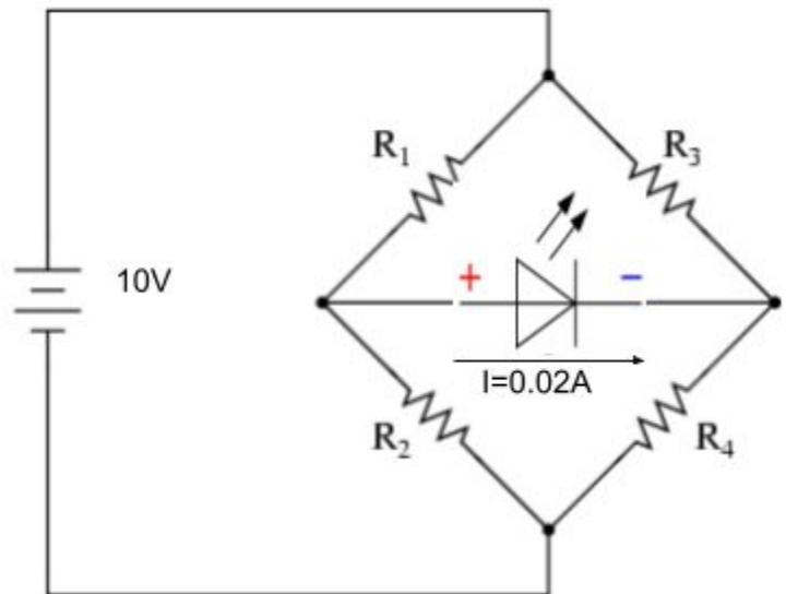
**Hint:** Assume that the voltage drop across LED and the current flowing through it are optimal:  $2\text{V}$  and  $0.02\text{A}$  respectively. Let current through resistor  $R_1$  be  $I_1$ . From here, find currents and voltages across other resistors.
