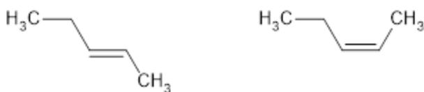
and these isomers have different chemical and physical properties. In addition, other hydrocarbons with the same empirical formula ( $C_5H_{10}$ ) can exist, so called cycloalkanes, cyclopentane, methyl cyclobutene and two isomeric dimethyl cyclopropanes:
