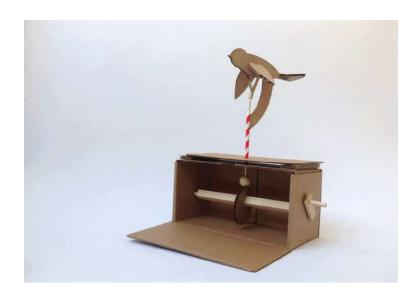
Ever wonder how wind up toys or animatronics work? Automata are moving sculptures that are powered by simple mechanisms, and change circular motion into vertical motion by using cams. In this workshop, you'll learn how automata work, experiment with mechanical motion, and build your own cardboard automaton with a custom scene. If you're interested in engineering, art, or just want to make a moving art piece, this workshop is for you!
